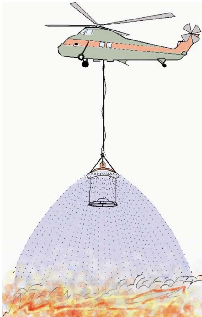
**Figure 4** – HELSY-high rate spray system in action
