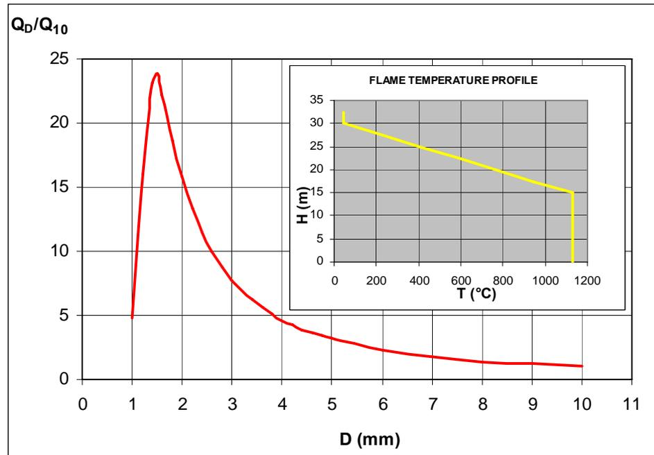
**Figure 3** - Ratio of the heat absorbed by uniform spray while passed through a hot flame surrounding with an assumed temperature profile to the referential spray heat absorption capacity
