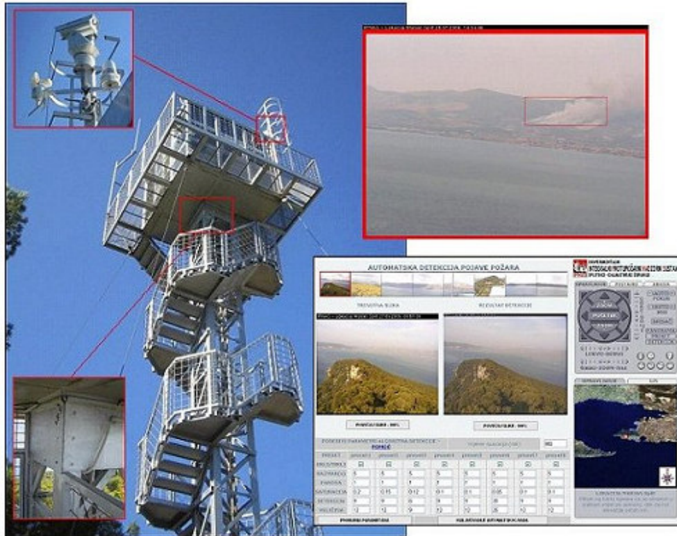
Figure 6 — Experimental forest fire monitoring station on Marjan hill (Split area) working during 2005 and 2006 fire season and two screens of iForestFire – intelligent Forest Fire monitoring system developed at the University of Split
