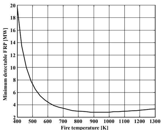
**Figure 10** – Minimum fire radiative power (FRP) detectable using SFIDE algorithm.
